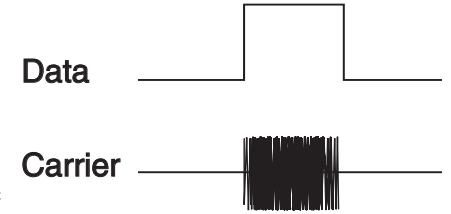
Figure 12: CPCA (AM) Modulation
